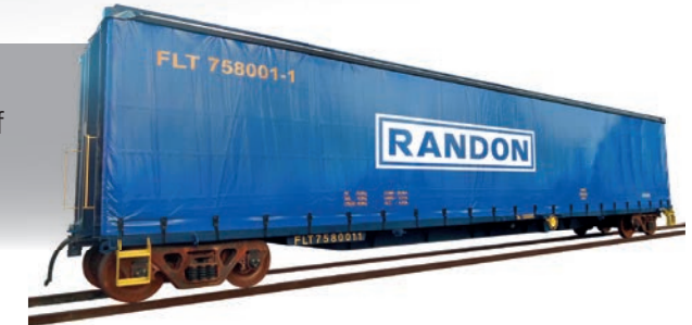
Sider Ideal for the transport of cement bags and other palletized loads.
